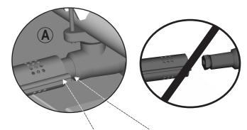
Correctly assembled burner tube and valve.
